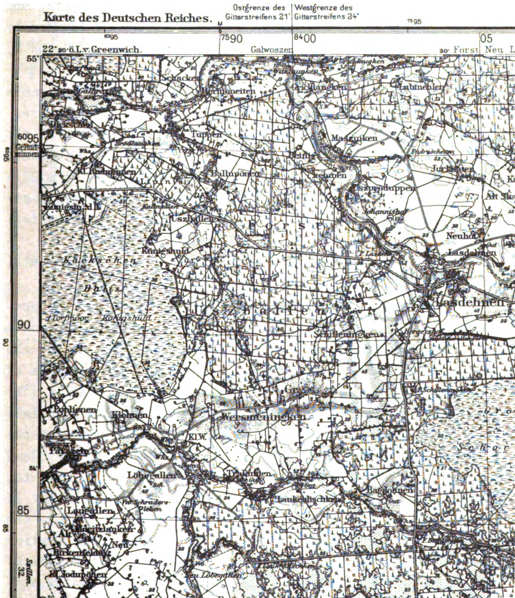
FIG. 15.--Section of map from Reichskarte Series, 1:100,000, Sheet 33. Note the boundary between grid zones, the numbering system, and the tick marks used to extend the grids of the two zones.
